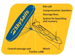
The towing kite of the SkySails propulsion system has an aero-dynamically optimised aerofoil-profile, comparable to the wing of an aeroplane. Thus the SkySail is also suited for fast vessels. It can easily be launched and recovered. The towing kite is made of a robust, weatherproof textile, can easily be stored and takes up little space on board.
