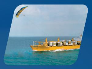
The system consists of a towing kite, an autopilot and wind-optimised route management.
